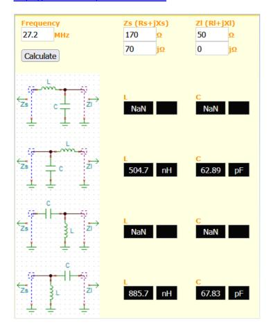
In this case option 4 is used. L consists of 820nH and 68nH in series. C is a 100pF trimmer capacitor.
