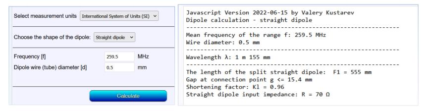
In this case the gap = 12mm. As a result the length of each element is 271.5mm.
